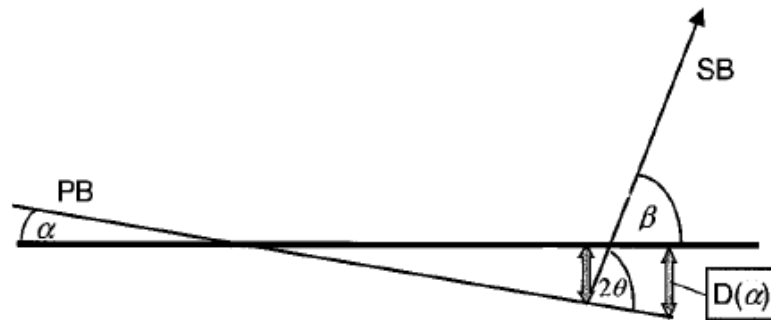
Figure 3 – Incidence and diffracted beams with respect to the sample surface
